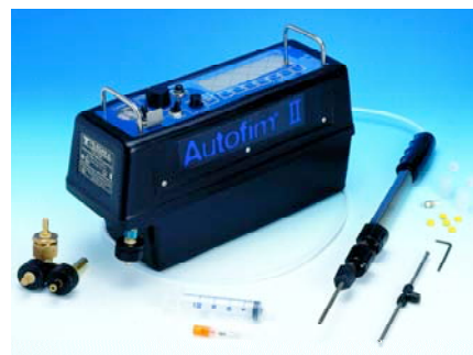
FID based instrument with built-in gas chromatograph can identify methane, benzene etc in ppm levels
