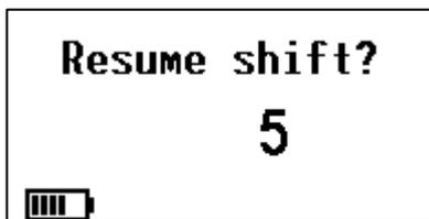
If a Gas-Pro is now being used by a new operator and the "TWA Resume" function is not required, **do not click the operator button**, and simply allow the countdown to expire. This will reset the STEL, TWA and peak values back to zero.
