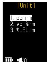
When the "3. %LEL·m" is selected in the upper right screen, the [Unit] screen shown on the right will be displayed. The lower explosion limit value indicated by the column density can be selected.
