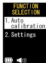
5. Automatic calibration will start, and for 2 to 3 minutes, the [AUTO CALIBRATION] screen shown on the right will be displayed.
