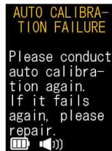
**CAUSE** Automatic calibration is not performed correctly.
