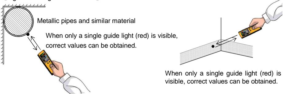
2. For a PE (polyethylene) pipe with a wall thickness of less than 10mm, please note that you may get wrong measurements if you keep pointing the laser directly at the PE pipe, because laser light penetrates through depending on its thickness.
