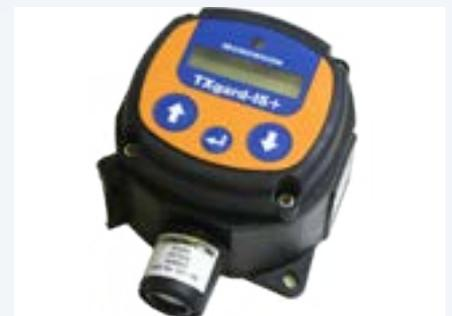
TXgard-IS+ is an Intrinsically Safe (I.S.), 2-wire, toxic and oxygen gas detector with local LCD display. A wide choice of sensors is available for use in a variety of applications. TXgard-IS+ is ATEX and IECEx certified for use in Zone 0, 1 or 2 hazardous areas, and also UL and cUL certified for use in Division 1 or 2 hazardous areas.
