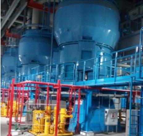
If coal is to combust efficiently in boilers, it must be pulverized into fine particles (100µm) before being placed in the boiler. A coal pulveriser is used to break pieces of coal down in this way.
